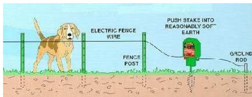
An electric fencing system presents a mental barrier to an animal rather than a physical barrier. Once an animal is shocked, it will respect the fence out of fear of being shocked again, even though it has not been harmed. The electric fence energizer produces an electrical pulse that travels through the lead-out wire into the wire(s). The electricity then flows through the animal's body into the soil and back to the ground rod which is connected to the energizer's ground terminal.
