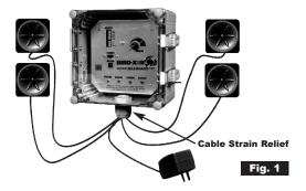
Prior to operation, route the speakers and power cables from their respective jacks on the control panel down through the cable strain relief in the lower part of the enclosure, as shown in Figure 1.
