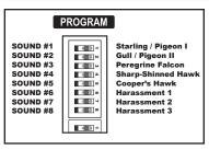
The Sound S e t t i n g Switches are the first eight switches in the switch array, and set the sonic (audio) sounds only.
